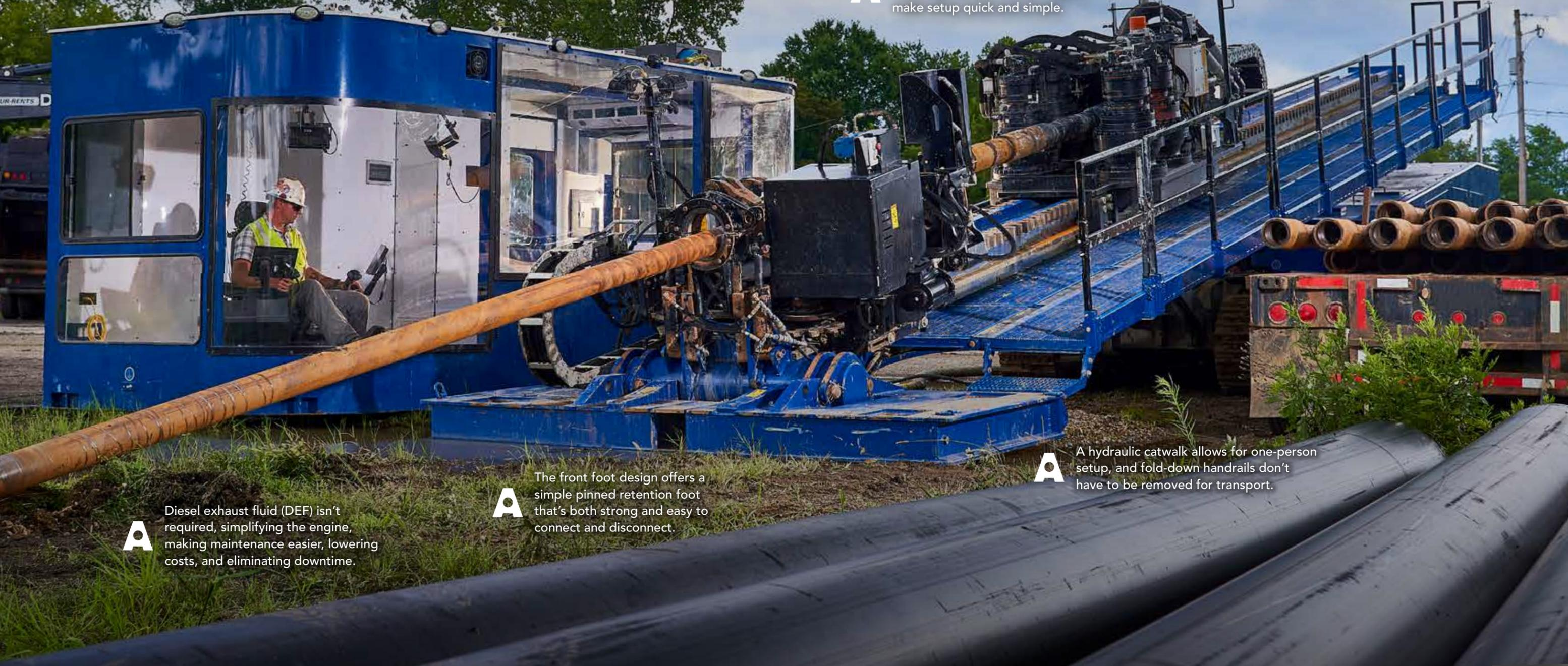
**A** Diesel exhaust fluid (DEF) isn't required, simplifying the engine, making maintenance easier, lowering costs, and eliminating downtime.
